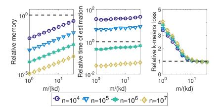
Relative time, memory and *k*-means risk of CKM with respect to *k*-means  $(10^0 \text{ represents the } k\text{-means result})$ . (*d* = 10)
