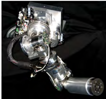
additional F/T sensor at the end-effector
